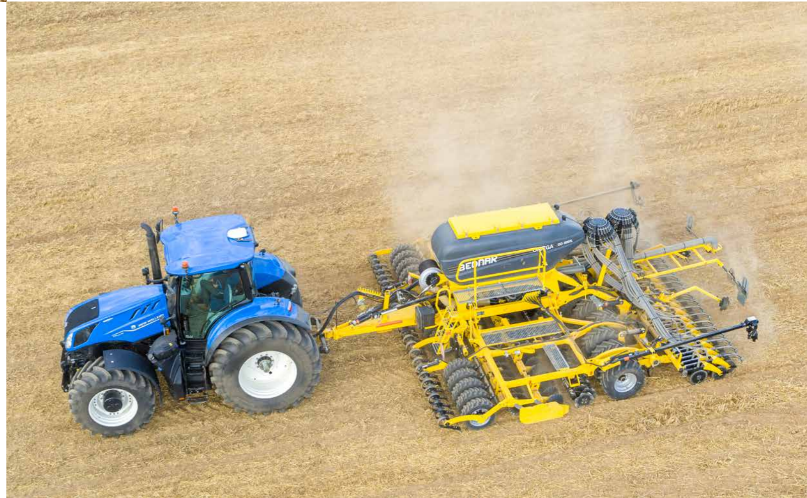
The independently mounted coulters work in the same line as the rear drill coulters.
