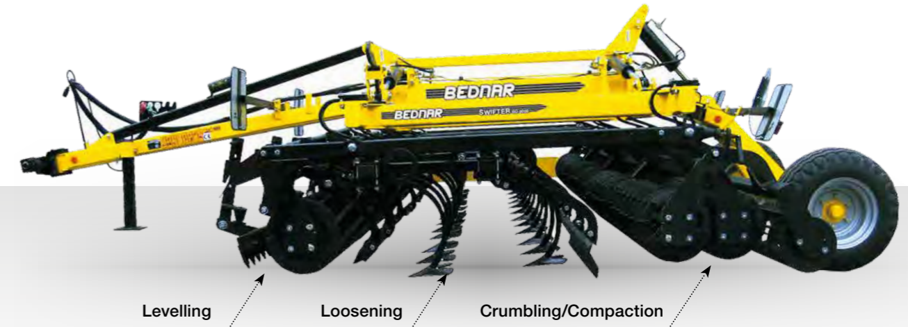
Working section with spring shares (SB-section)
